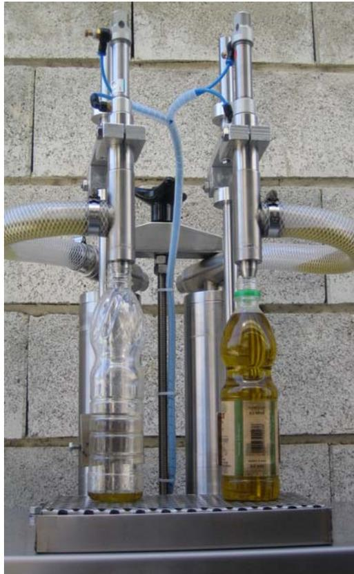
Nozzle system ensures cleanliness and accurate dosing.
