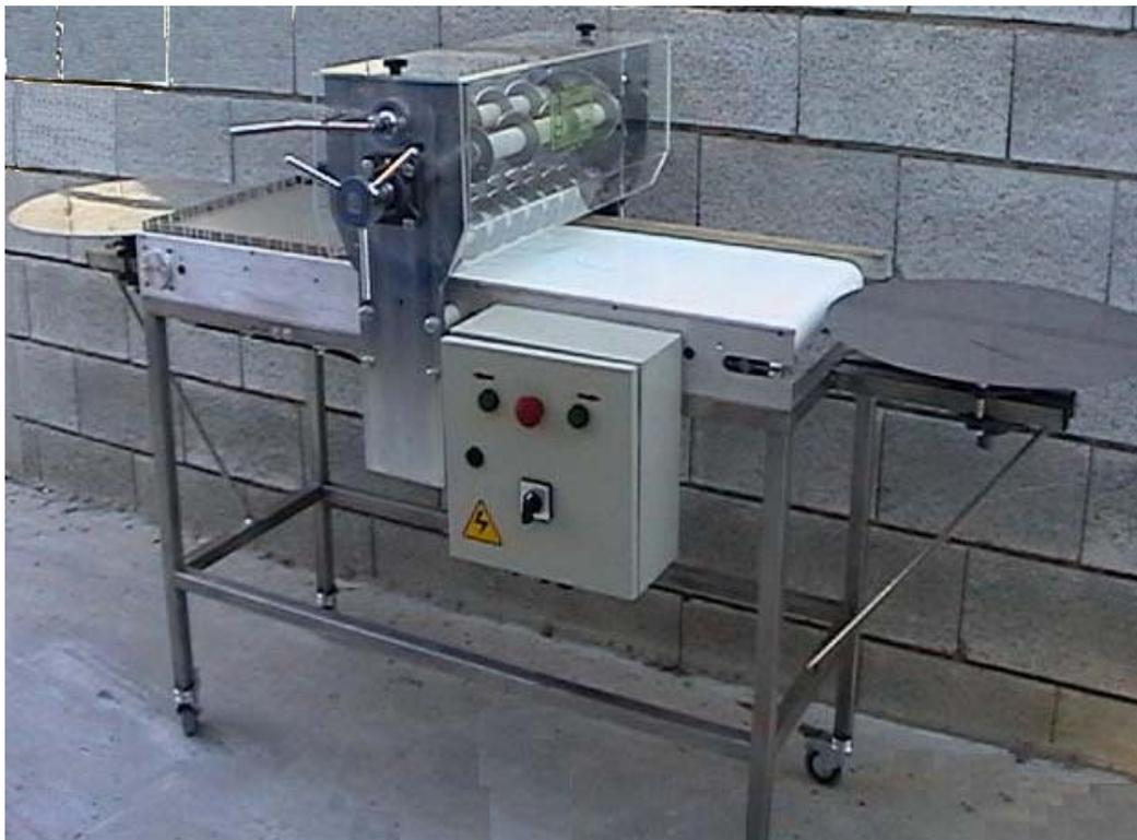
This machine was designed in order to reduce the time of cutting coconut sweets in rectangular shape.
